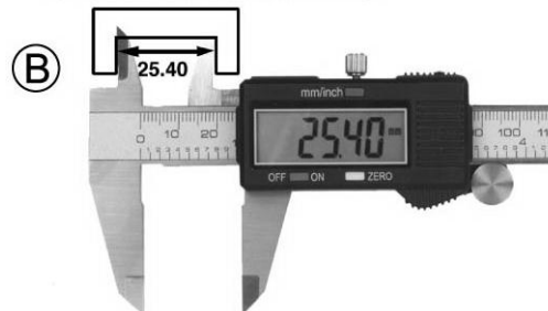
B. Measuring between inner surfaces
